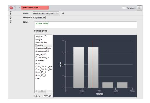
Fiber Shape Statistics internally reconstructs a labeled fiber data object from a grayscale image and a mask by converting the input spatial graph to a binarized representation (using the module Convert Geometry To Label) and growing it within the mask. This representation is then used to calculate the volume fraction of each fiber and deduce various statistics. The fiber shape statistics are the following:
