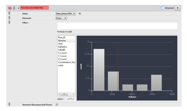
This module generates a new pore network model containing only the pores and throats resulting from this filtering. An option allows removal of all the disconnected pores in a second process.
