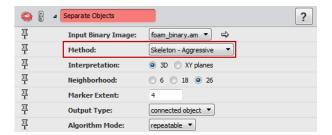
This method generates a label field using a separation algorithm based on watershedding and skeletonization, which carefully separates pores at throat centers.
